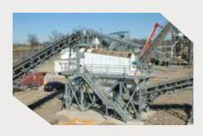
The rotating screens manufactured by Tecno-Beton are characterised by high strength which, associated with very simple use, makes them perfect to use as pre-screens to prepare material for subsequent crushing and sorting steps. Encapsulated in a screened structure, which makes moving parts inaccessible, they can host screen surfaces in rubberised sheet metal or polyurethane, based on screening needs.
