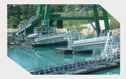
Tecno-Beton manufactures the entire range of floating conveyors necessary to transport aggregates extracted by the dredge onto the ground. Based on configuration and use, they are divided into:
