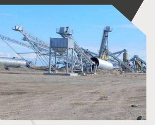
H series conveyors: manufactured in thick sheet metal, with the sides shaped to facilitate conveyance of material accidentally falling into the upper section towards the outside, they are designed for medium-long distances. The components of the conveyor are made of interchangeable modular elements. Also for this series there are accessories such as side rails, stone traps, sunshades, wind-proof ribs, gangways, drainage covers, etc.
