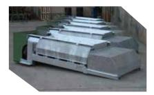
These feeders are manufactured using a short conveyor with a low profile. Completely edged to avoid material falling from the sides, they are applied under silos or hoppers for material extraction. Structure completely galvanised with interchangeable, anti-wear rubber rails. Servo-ventilated engine installed for use with inverter.
