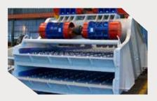
Tecno-Beton Impianti manufactures horizontal dewatering screens, normally used to dewater sand arriving from the washing and sorting process. The screening surface is typically manufactured in polyurethane drainage panels and motion is driven by two synchronous electric vibrators.
