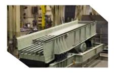
MACHINES SUITABLE FROM SEPARATING FINE PARTICLES FROM QUARRY DEBRIS, THEY ARE INSTALLED UPSTREAM OF THE PRIMARY CRUSHERS AND UNDER THE LOADING HOPPERS.
